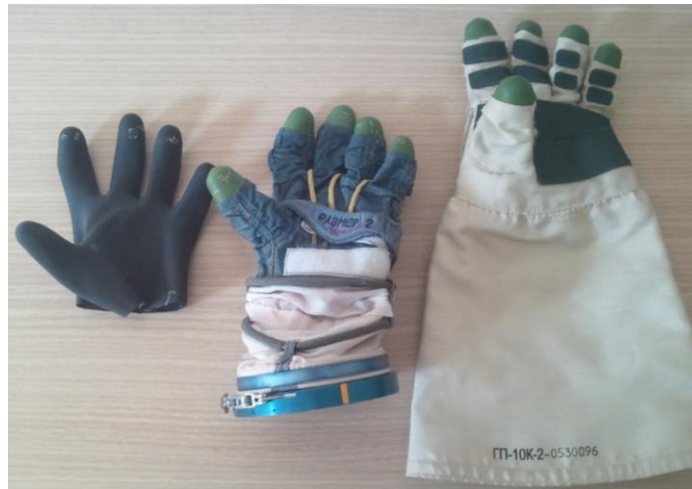
Figure 1. Orlan-DM glove used for testing. Inner rubber glove (a), EVA glove (b), and outer TMG (c).
