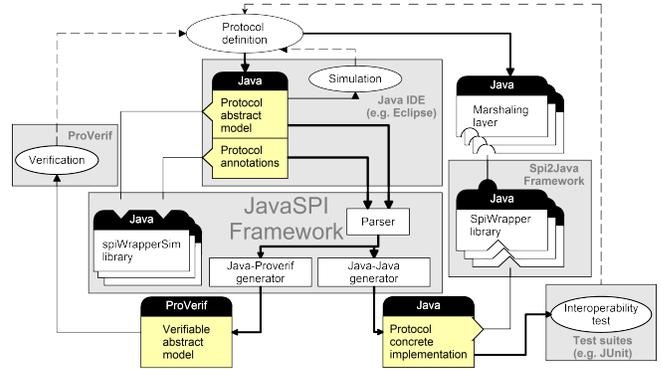
Figure 1. The complete workflow provided by JavaSPI.
