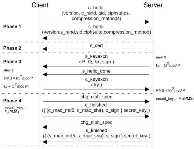
Figure 3. SSL message exchange in the selected scenario.
