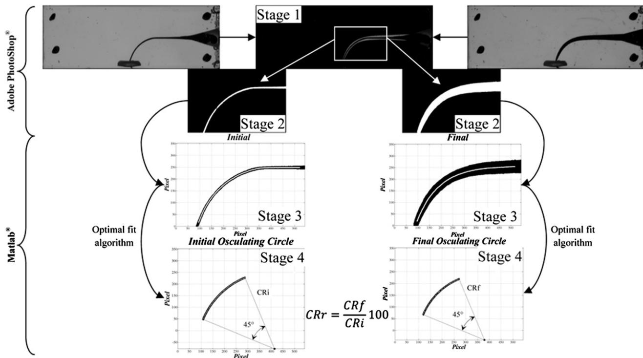
**Figure 1.** Scheme to determine the CRr parameter.
