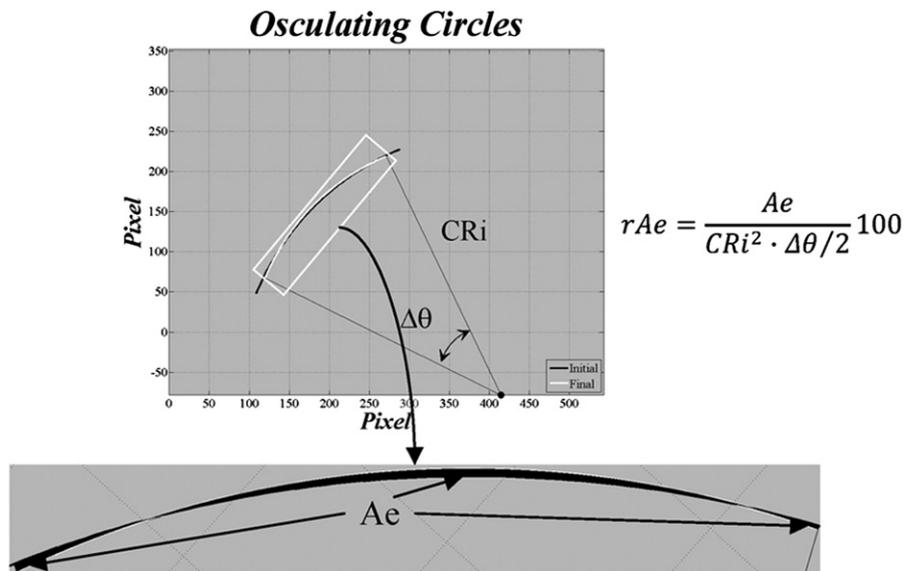
**Figure 2.** Scheme to determine the rAe parameter.
