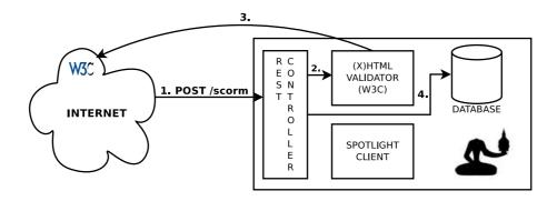
**Fig. 4.** Workflow describing the upload of a SCORM package in Zenaminer: 1. a SCORM package is received from a client; 2. (X)HTML files are forwarded to the validator; 3. (X)HTML files are validated by sending requests to the offical W3C validator; 4. if all documents are valid, the SCORM package is stored to the database.
