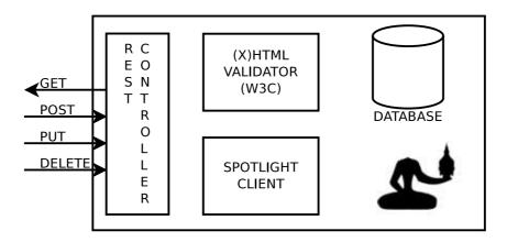
**Fig. 2.** Zenaminer architecture. The REST controller is the interface between Zenaminer and the Internet; the W3C validator is used to check that imported (X)HTML files are well-formed; the Spotlight client provides automatic annotation; the database stores imported SCORMs together with comments and annotations.
