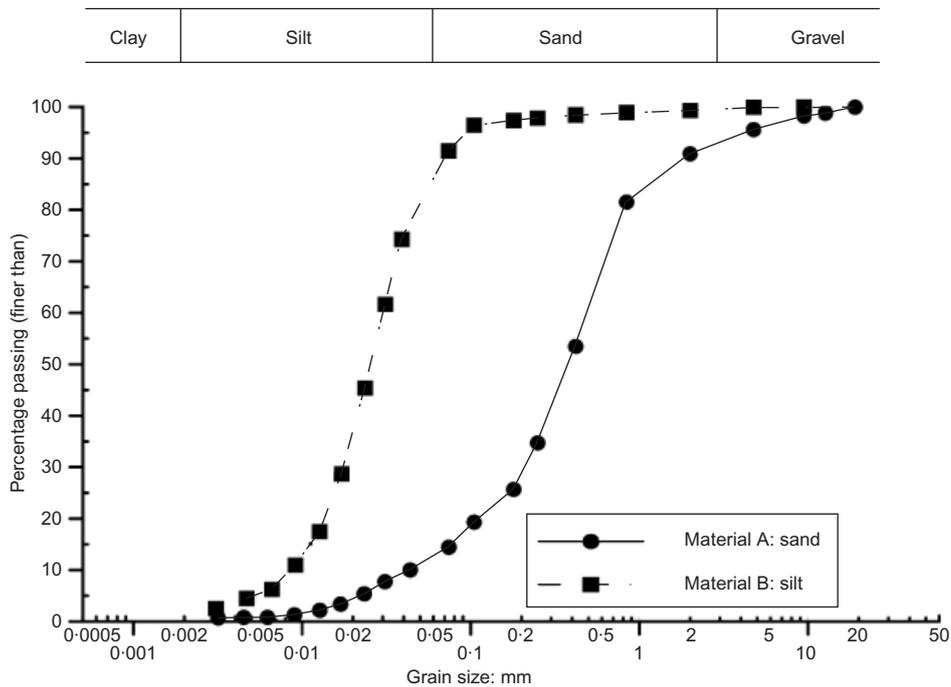
Fig. 3. Grain-size distribution of the sand and silt specimens
