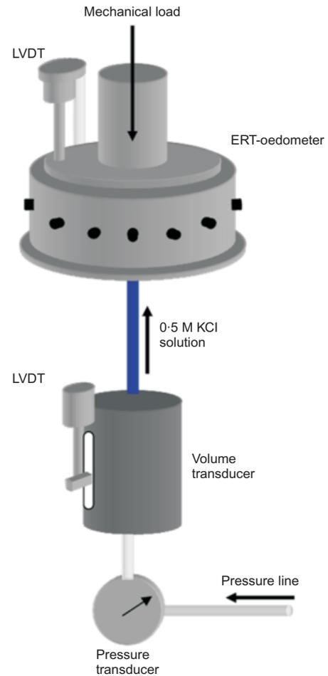
**Fig. 2. Experimental assembly (LVDT, linear variable differential transducer)**
