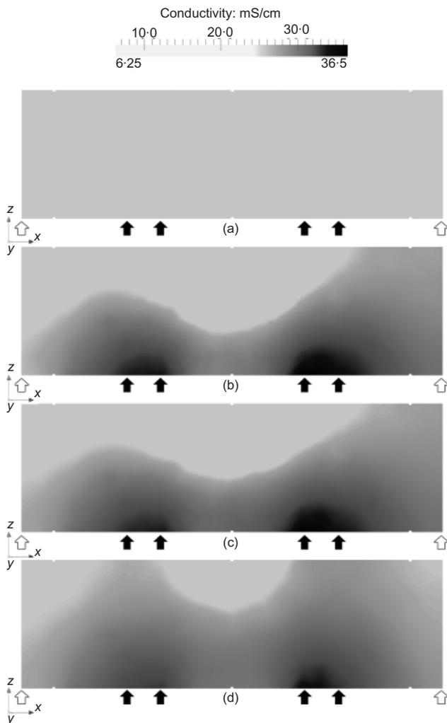
Fig. 8. Test 1A: Time evolution of electrical conductivity over a longitudinal cross-section: (a)  $t = 0$  min; (b)  $t = 10$  min; (c)  $t = 110$  min; (d)  $t = 3000$  min (arrows indicate drain positions)
