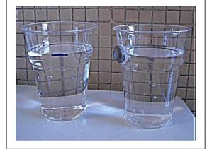
Fig.2 Two cups can be used to repeat the measure of volumes as described by Vitruvius. On the right, we see the cup with a hole, with a plastic ring glued about it. It simulates the vessel of a water-clock
