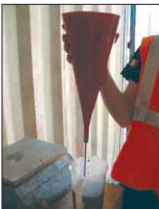
Figure 4. Execution of Marsh cone test.
