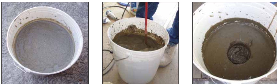
Figure 3. Phases of preparation of the hardened grout samples.
