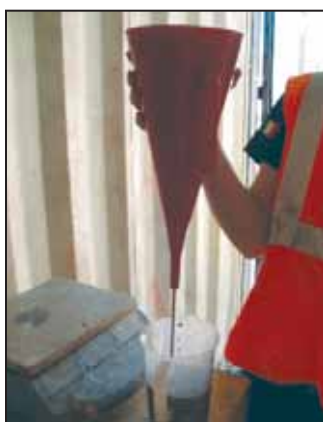
Figure 4. Execution of Marsh cone test.
