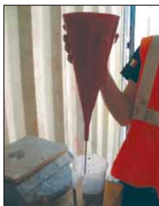
Figure 4. Execution of Marsh cone test.
