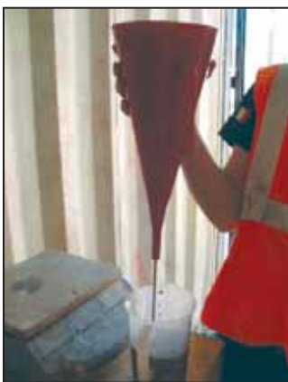
Figure 4. Execution of Marsh cone test.
