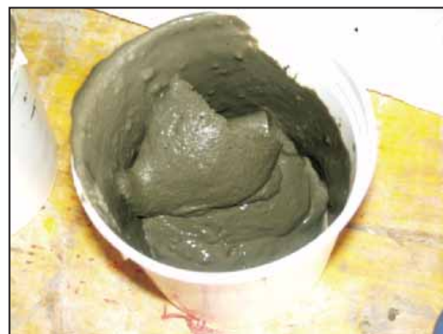
Figure 5. Grout mix after hardening.
