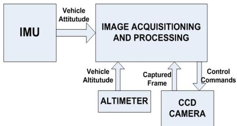
Figure 4. Block Diagram of Sensor Integration for Imaging
