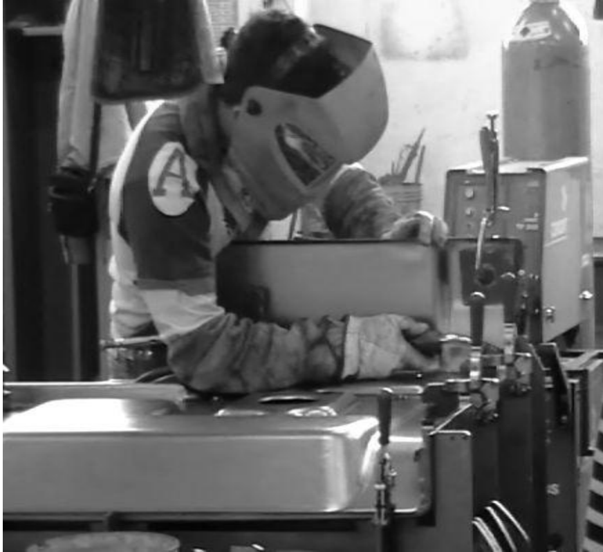
FIGURE 2. The still from a video made by the authors. The welder is going to start the welding of a complex joint in a hard to reach area on the workpiece
