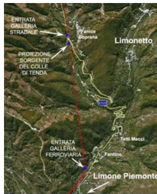
Fig. 2: Detail showing the area under examination. The aerial view shows the entrances to the two tunnels, the projection of the Sorgente di Tenda on the natural surface and the route of the rail tunnel
