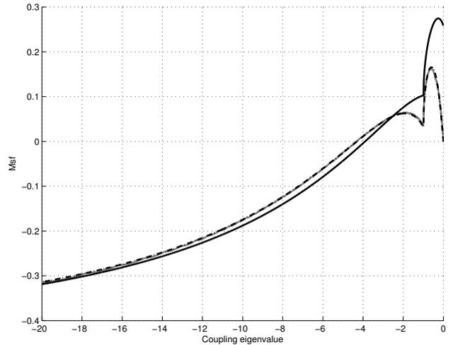
Figure 4: MSF for the Chua circuit: black lines are obtained with the HB approach described in Sec. 3 with  $K = 1$  (solid),  $K = 3$  (dashed), and  $K = 5$  (dotted), whereas the solid grey line is obtained in the time-domain.
