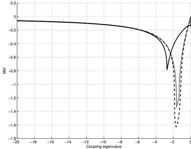
Figure 3: MSF for the Van der Pol oscillators: black lines are obtained with the HB approach described in Sec. 3 with  $K = 1$  (solid),  $K = 3$  (dashed), and  $K = 5$  (dotted), whereas the solid grey line is obtained in the time-domain.
