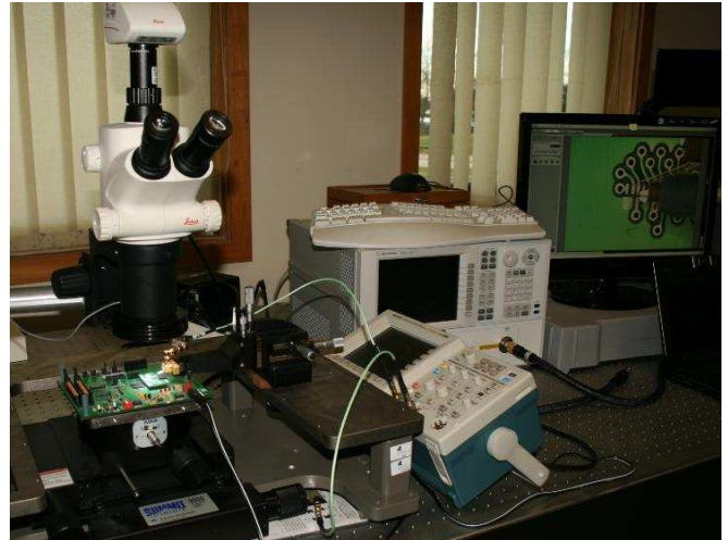
Fig. 11. Image of the measurement workbench, while probing an I/O buffer output of the external MM.
