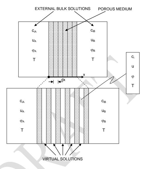
Figure 3. Conceptual scheme of the Spiegler and Kedem (1966) model. Subscript A and B refer to the electrolyte solution reservoirs on the left and on the right of the thermodynamic discontinuity, that represents the membrane. Symbols:  $c_i$  = ion concentration of the i-th ion; u = hydraulic pressure;  $\phi$  = electric potential; T = absolute temperature.
