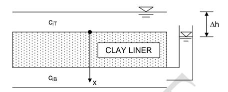
Figure 1. Reference problem representing a horizontal clay barrier separating two electrolyte solutions containing different ion concentrations. Symbols:  $c_{iT}$  = concentration of the i-th ion in the solution at the top of the liner;  $c_{iB}$  = concentration of the i-th ion in the solution at the bottom of the liner;  $\Delta h$  = difference in the hydraulic head between the top and bottom electrolyte solutions; x = spatial coordinate.
