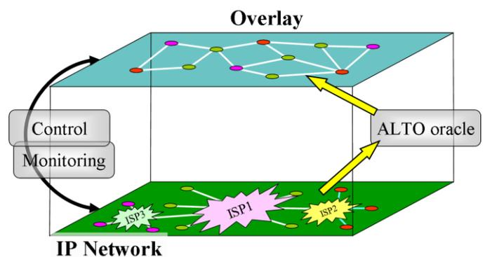
**Figure 1: NAPA-WINE Vision - IP routers and overlay nodes (peers) cooperate through monitoring and control capabilities, and ALTO interaction to optimize performance and network usage**
