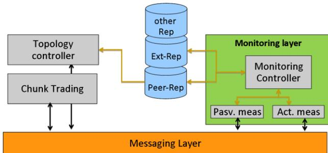
Figure 5: Detailed architecture of the monitoring modules.
