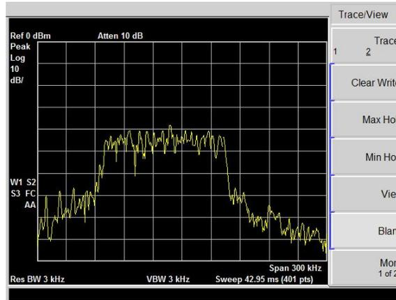
**Fig. 4.** Bandwidth of OFDM signal created by USRP.
