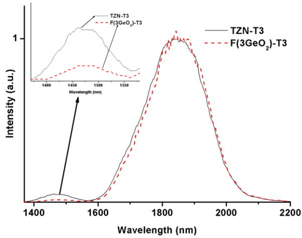
Fig. 6b) Emission spectra of TZN vs. FTG for 3 mol % Tm<sup>3+</sup>.
