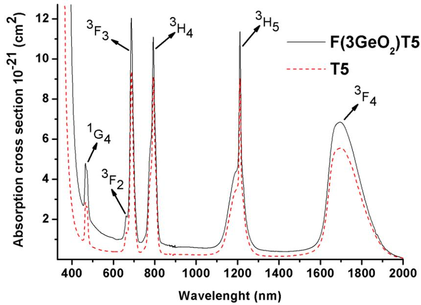
Fig. 1. Absorption cross section of TZN – T5 and F(3GeO<sub>2</sub>) T5 samples.
