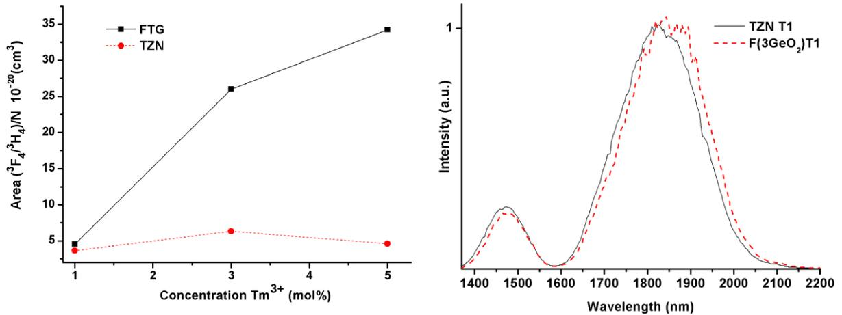
Fig. 5. Area of the peak emission ratio over ion concentration for three different samples of FTG and TZN hosts. Fig. 6a) Emission spectra of TZN vs. FTG for 1 mol % Tm<sup>3+</sup>.
