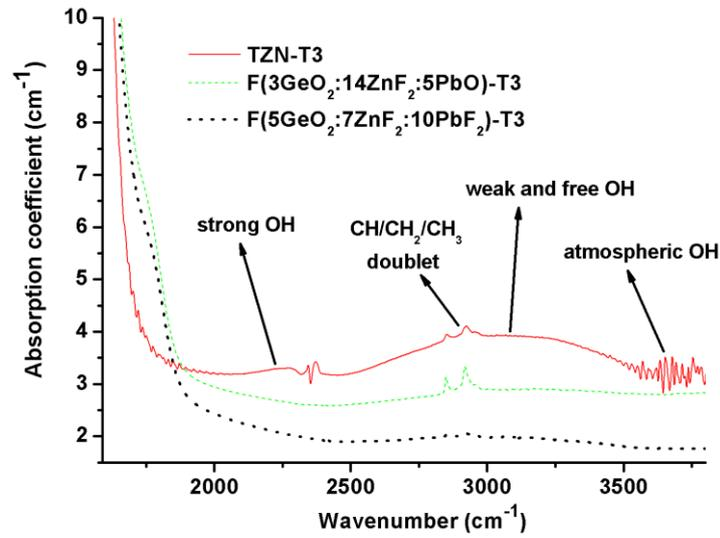
Fig. 4. FTIR spectra of TZN, F(3GeO<sub>2</sub>:14ZnF<sub>2</sub>:5PbO) and F(5GeO<sub>2</sub>:7ZnF<sub>2</sub>:10PbF<sub>2</sub>) doped with 3 mol% of Tm<sup>3+</sup>.
