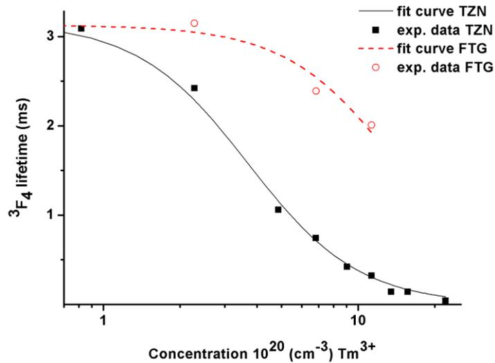
Fig. 7. Lifetime values decay from <sup>3</sup>F<sub>4</sub> level for various dopant concentrations
