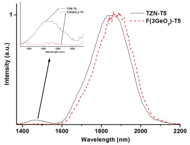
Fig. 6c) Emission spectra of TZN vs. FTG for 5 mol % Tm<sup>3+</sup>.
