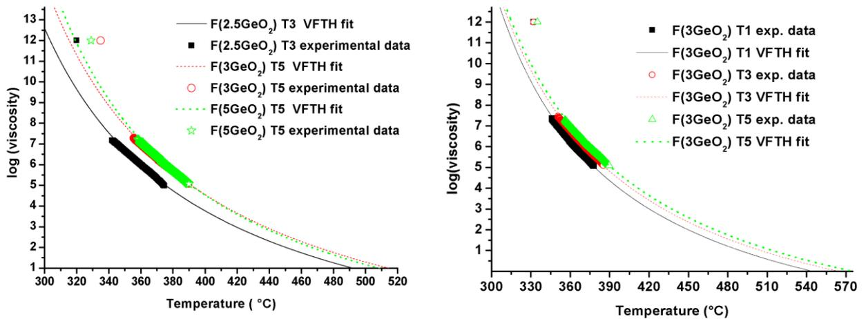
Fig. 2a) Viscosity curves of FTG glasses for different GeO<sub>2</sub> content.
