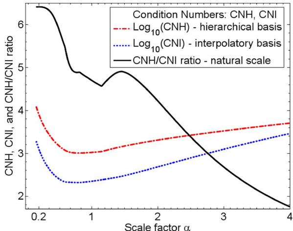
Fig. 2. Individual element  $\mathbf{T}$ -matrix condition numbers for the hierarchical (CNH) and the interpolatory (CNI) vector basis of order 2.5 obtained by considering tetrahedral cells of different height  $\alpha \sqrt{6} \ell/3$ , but with the same equilateral base of edge-length  $\ell$ .
