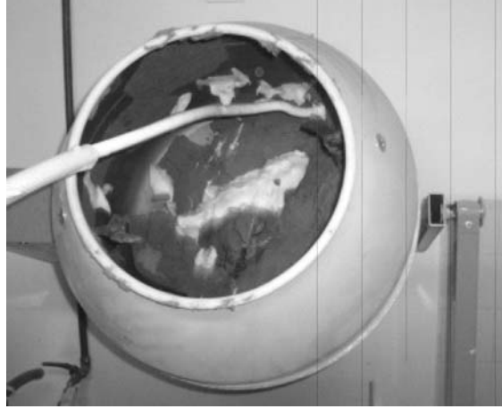
Fig. 2. Soil conditioning in the mixer bowl
