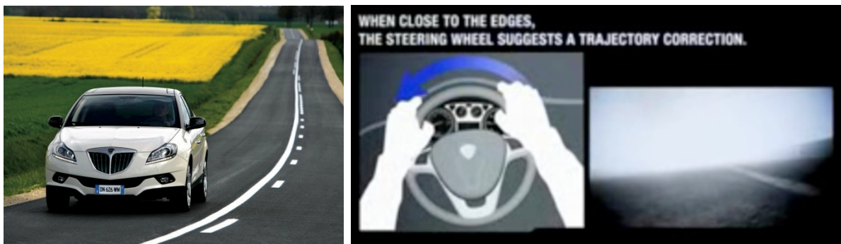
Figure 1. Lancia Delta and the LDW system
