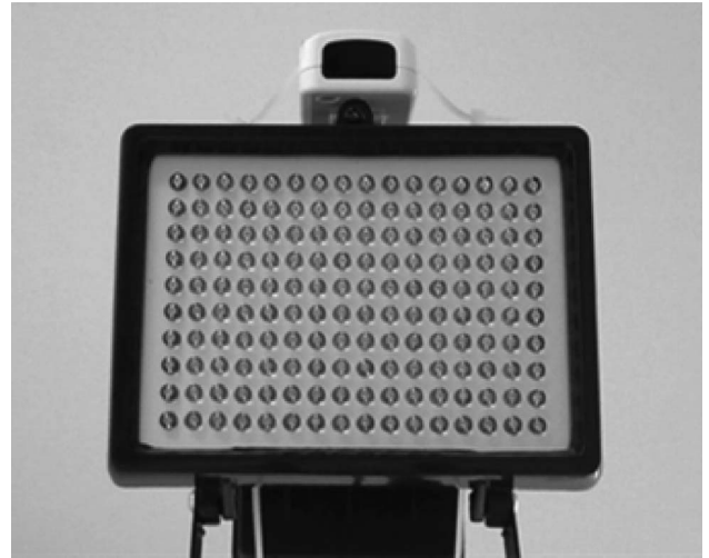
Figure 4. Main components of the IR-based sensor network: an IR camera is coupled with an IR LED array to locate passive retro-reflective targets.
