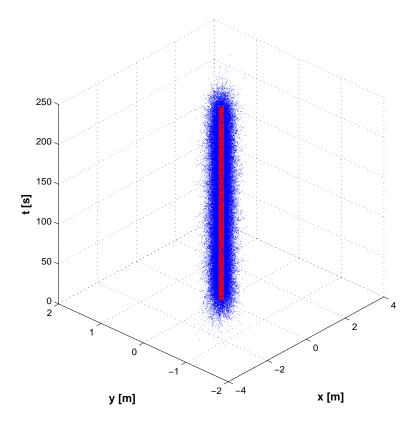
FIG. 1: Reconstructed world-line of an user at rest. The straight vertical line is the expected result; the scattered blue points are the reconstructed positions obtained applying our method with a nanosecond Gaussian noise in the input. The RMS dispersion is of the order of less than 40 cm. The greater dispersion of the x coordinates with respect to y is due to the anisotropic distribution of the sources in the sky.
