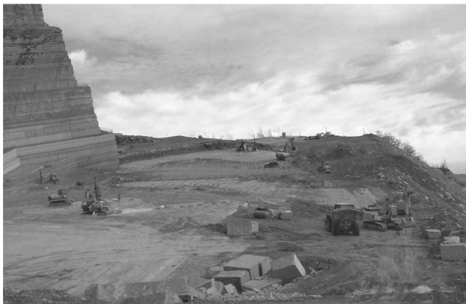
Fig. 3. View of the machines on the quarry yard exposed to rock-fall phenomena
