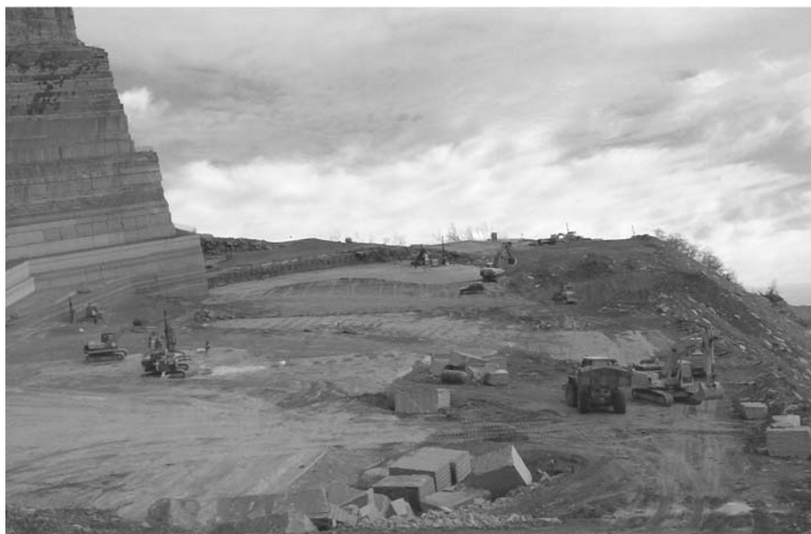
Fig. 3. View of the machines on the quarry yard exposed to rock-fall phenomena
