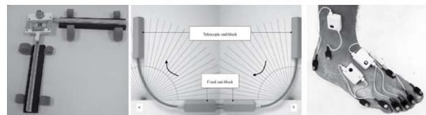
Fig.13. Electro-goniometer sensor [18]
