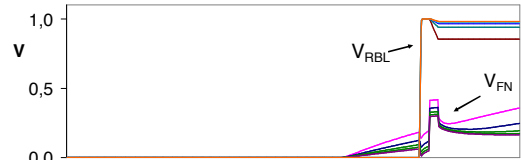
Figure 16 Incorrect readout of Q=0 due to O2 with resistance higher than 300MΩ. The write and read actions are the same as in Figure 14.
