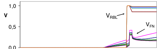
Figure 16 Incorrect readout of Q=0 due to O2 with resistance higher than 300MΩ. The write and read actions are the same as in Figure 14.
