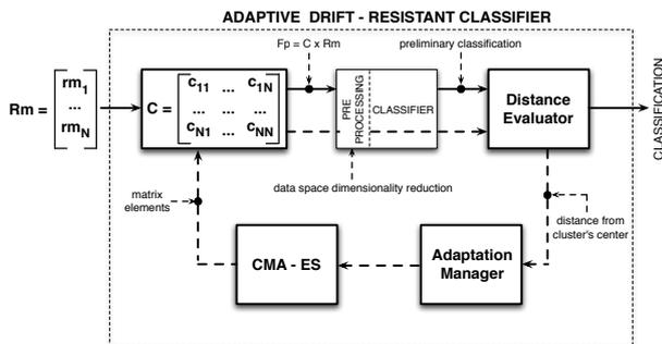
**Figure 1: Conceptual architecture of the drift corrector**
