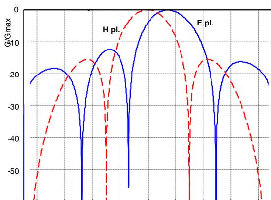
Fig. 5: Radiation patterns of the reflectarray on the symmetry (vertical) plane (E plane, solid curve) and in the H plane (dashed curve).
