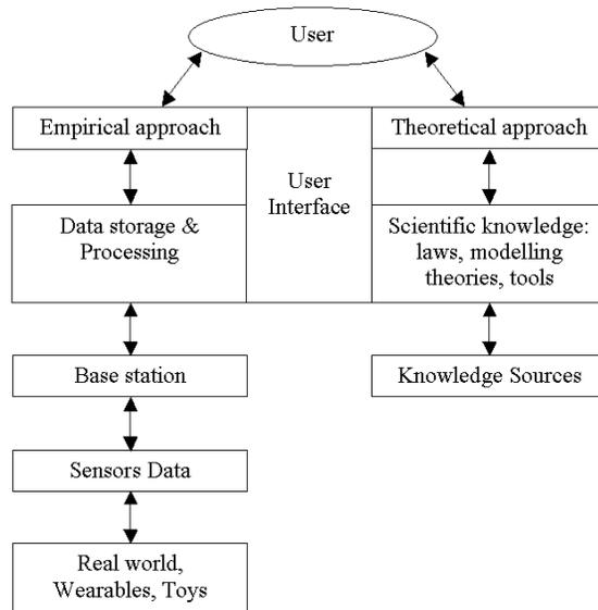
The LoT system should be seen as a way to increase the observation capabilities of the user. Through the empirical interface, the user gains a view of the world from scientific instruments that surpasses human senses in sensitivity and range; through the theoretical interface, the user engages scientific modelling to his thinking.
