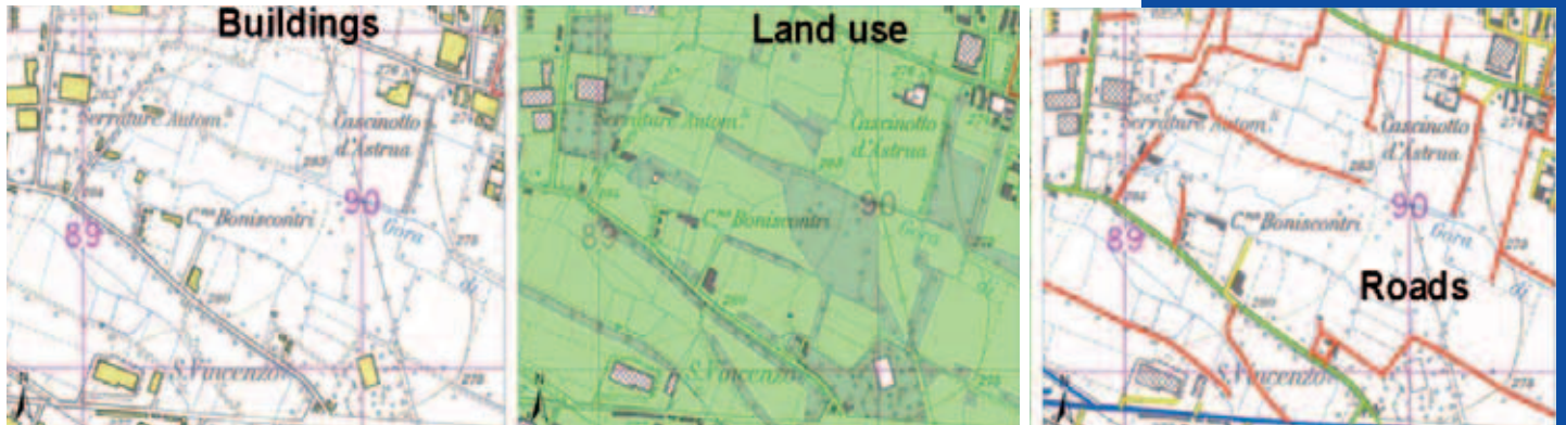
Fig. 2 Landscape features (roads, buildings, land use) vectorized from the original raster maps. Fig. 3 Methodology for representing the Landscape Quality and its difference in time as space dependent functions (raster maps of indices).
