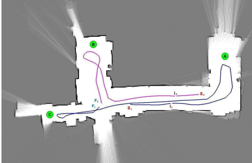
Figure 11: Map estimated through RBPF multi robot SLAM during experimental test at Politecnico di Torino. The corridor length is about 20 m whereas the particle set size was 100.
