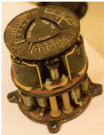
Figure 7: A triple indicator from the fallen aircraft dashboard.
