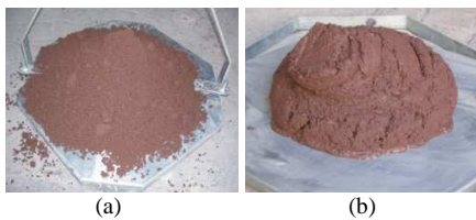
Fig. 7: Example of the behavior of the Rome Pozzolanic soil: Comparison of the slump tests of natural soil (a) and the conditioned one (b) with FER = 16, FIR = 25% and water content = 10%
