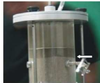
Fig. 3: Photograph of the permeameter during the test. The arrow indicates the position reached by the water inside the sample when the photograph was taken
