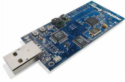
Figure 3: Tmote Sky wireless sensor module
