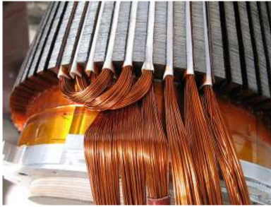
Fig. 7: First Prototype: windings particular
