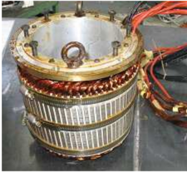
Fig. 8: First Prototype: stator complete
