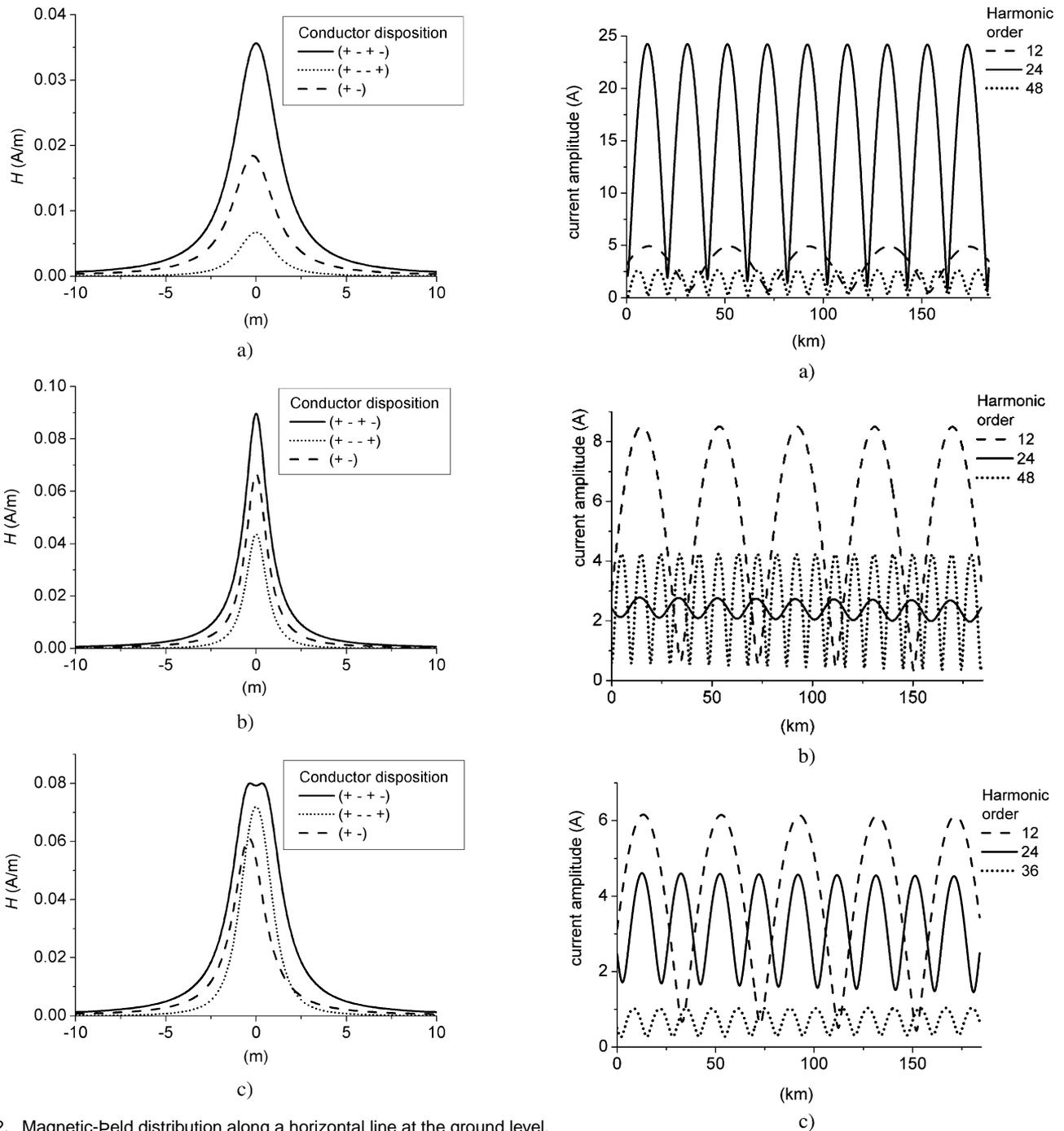
Fig. 2. Magnetic field distribution along a horizontal line at the ground level, corresponding to a current of 1 A. The origin is placed at the system center. (a) Configuration #1 in the highway. (b) Configuration #2 in the viaduct. (c) Configuration #3 in the tunnel.
