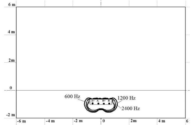
Fig. 10. Bounds of the regions where the magnetic field is higher than the EMC limit for information-technology equipment considering the tunnel laying with a shield composed of two opposed U-shaped ferromagnetic laminations.
