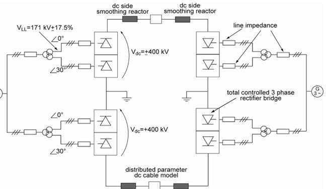
Fig. 1. Model of the analyzed HVDC system (line A or B).
