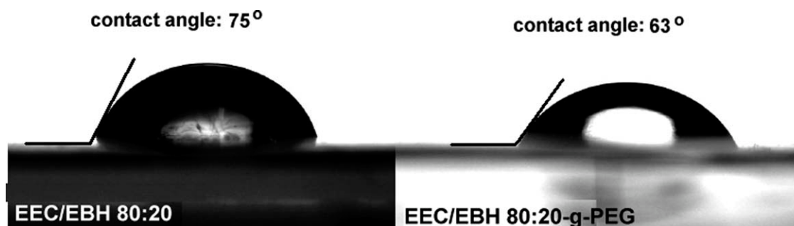
FIGURE 6 Static contact angle of water on the EEC/EBH 80:20 cured film ( \theta value 75^\circ ) and static contact angle of water on EEC/EBH 80:20- g -PEG ( \theta value 63^\circ ).
