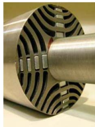
Fig. 4 – Permanent-Magnet Assisted Synchronous Reluctance (PMASR) rotor during motor assembling.
