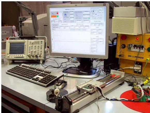
Fig. 6. LTPMSM prototype used for the tests.
