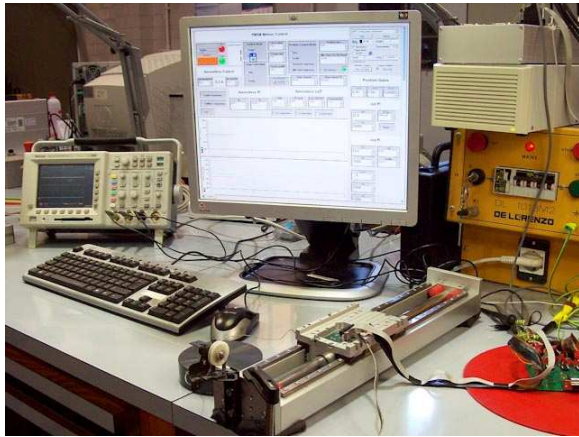
Fig. 6. LTPMSM prototype used for the tests.
