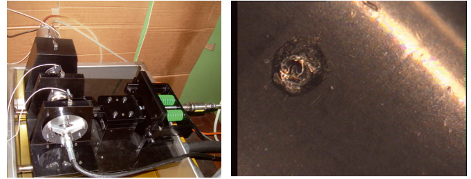
Fig. 2. Test rig (on the left) and damage on the rolling element after 50 h of testing (on the right).
