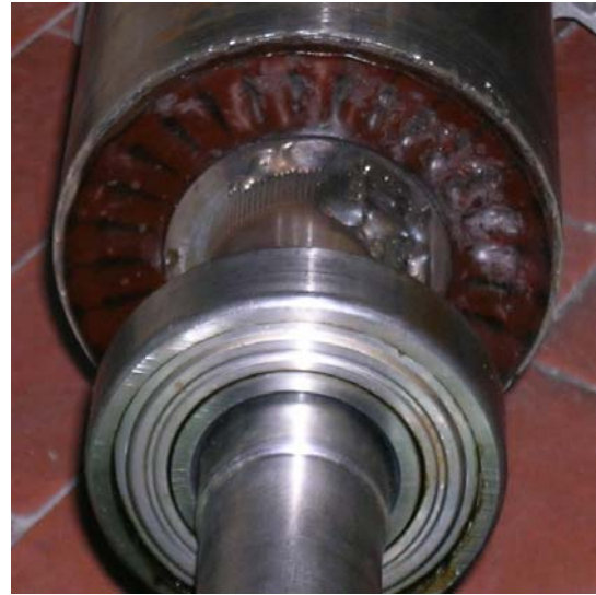
Fig.1: Rotor prototype with rubber cage
