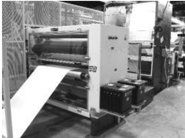
Figure 9.3 The universal system provides superior treatment levels, with elimination of film wrinkling and backside treatment
