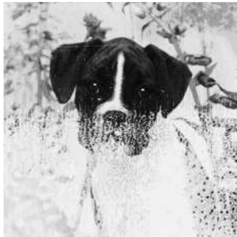
Figure 5.6 Beneficial effect of having sufficient substrate tension is shown in the figure. In the upper part the adhesion is perfect. In the lower part without treatment is instead highly ink defective.
