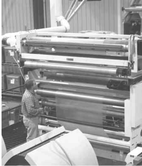
Figure 5.3 Inspection of a universal treater, the most common surface treater used to increase the surface properties of substrates before printing or converting.
