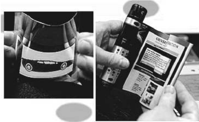
Figure 10.2 Flexible displays. The display can rolled-up in the control device.
