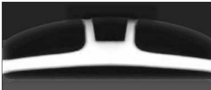
Figure 2.1 A homogeneous discharge between the two electrodes of an APT system.
