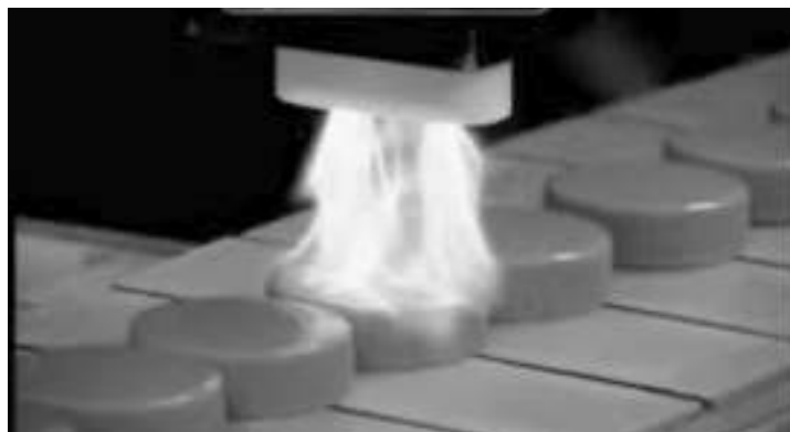
Figure 1.2 From sharp electrodes, discharges go toward the surface. With a suitable geometry, it is possible to treat the surface of two- and three-dimensional objects.
