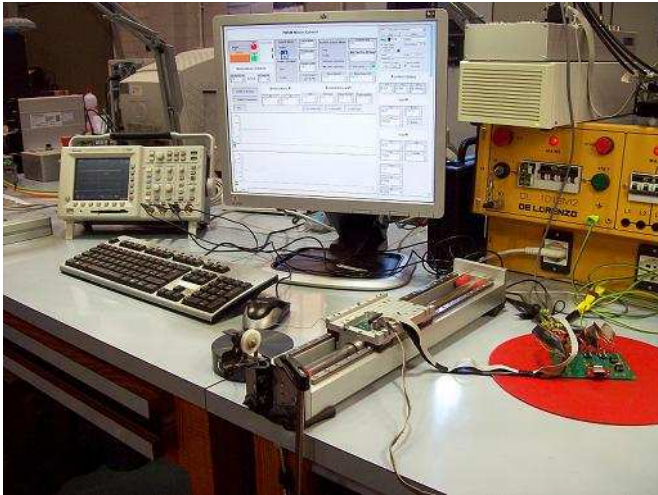
Figure 10. LPMSM prototype used for the tests.
