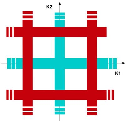
FIG. 3: Scheme of the filter CROSS that can be used as i) a high-pass filter: the wave-numbers under a certain threshold are partially removed, see (4) (region in blue in the  $k_1, k_2$  wavenumber plane), ii) both a band-pass and a low-pass filter: the wave-numbers inside a range, or above a certain threshold, are cut, see (5-7) (region in red).
