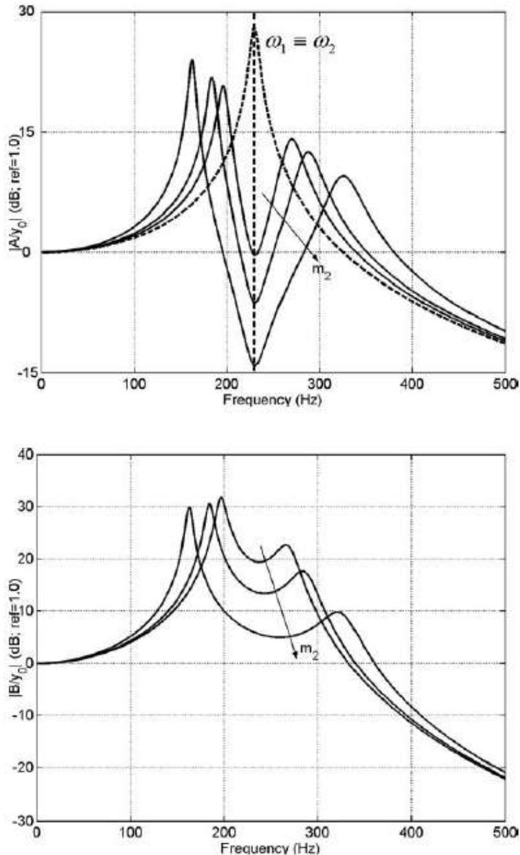
**Fig. 2** Transmissibilities of the dynamic absorber with  $m_2$  increasing. (a) Solid lines:  $A/y_0$ ; dashed line: FRF of the original sdof system; (b)  $B/y_0$ ;  $k_1 = 1.26 \times 10^5$  N/m,  $m_1 = 0.06$  kg,  $\omega_2 = 230$   $2\pi$  rad/s,  $m_2/m_1 = 1/10, 1/5, 1/2$
