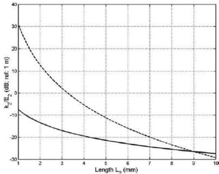
Fig. 4 Shear (solid line) and bending (dashed line) stiffness of the absorber with  $m = R_I/R_E = 0$
