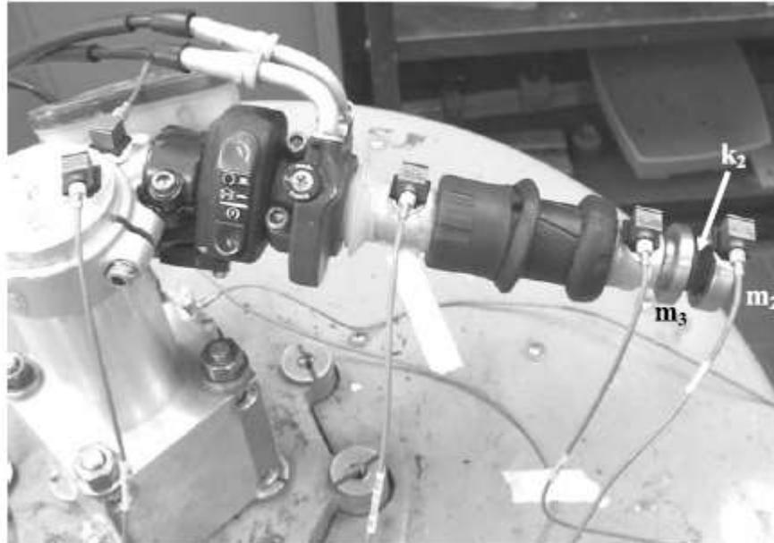
Fig. 9 The handle with the proposed vibration absorber
