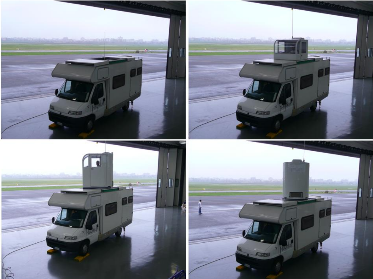
Figure 3: Pilot cabin movement system in the Mobile Ground Station
