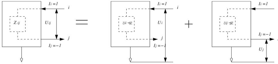
FIG. 1. The computation scheme of equivalent impedance.
